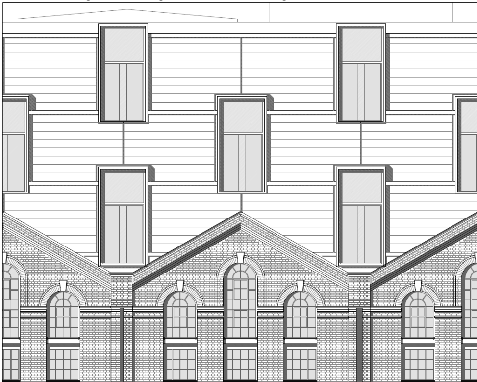
Figure 3: Original Dormer Design (Rear Elevation)
